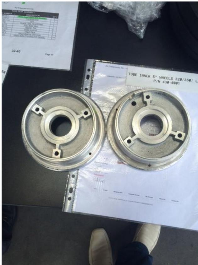
NAME: Nose Gear Wheel with Bearings
